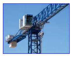
The hoist mechanisms include the *Effi-Plus* System, which improves up to 70% the speed of hoist and descend movements. With this system, the productivity during hoist operation is improved up to 27%, without any increase in power or electricity consumption.
